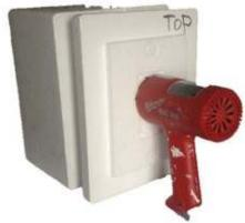
To stop heat from escaping around the sides we acquired a Styrofoam cooler (courtesy of Jeffrey Oda, USF Dept of Biology).
