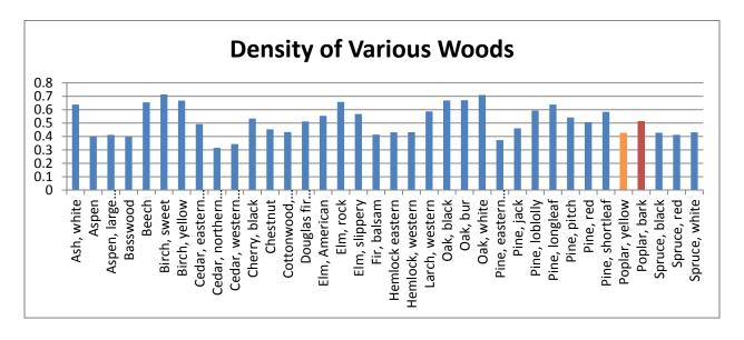
Then looking at various building materials such as fiberglass insulation (0.032 g/ml) and comparing them with the density of various woods, fiberglass' density is proven to be quite low and wood's density is high. Again notice how large poplar bark's density is considering its R-value as well. Since density is directly related to thermal mass, poplar bark can retain a significant amount of heat within itself, thus reducing heat loss enormously.
