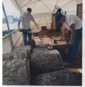
The bark has to be properly stripped from the wood and dried in a kiln before it can be used as a shingle.
