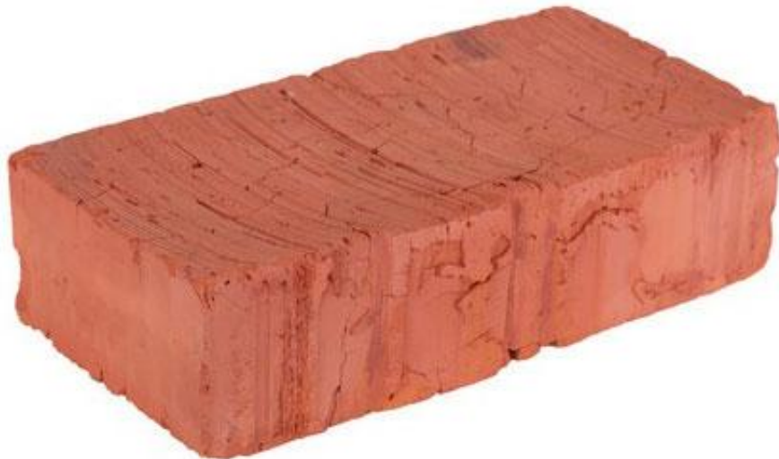
Brick ( clay, shale, water)
