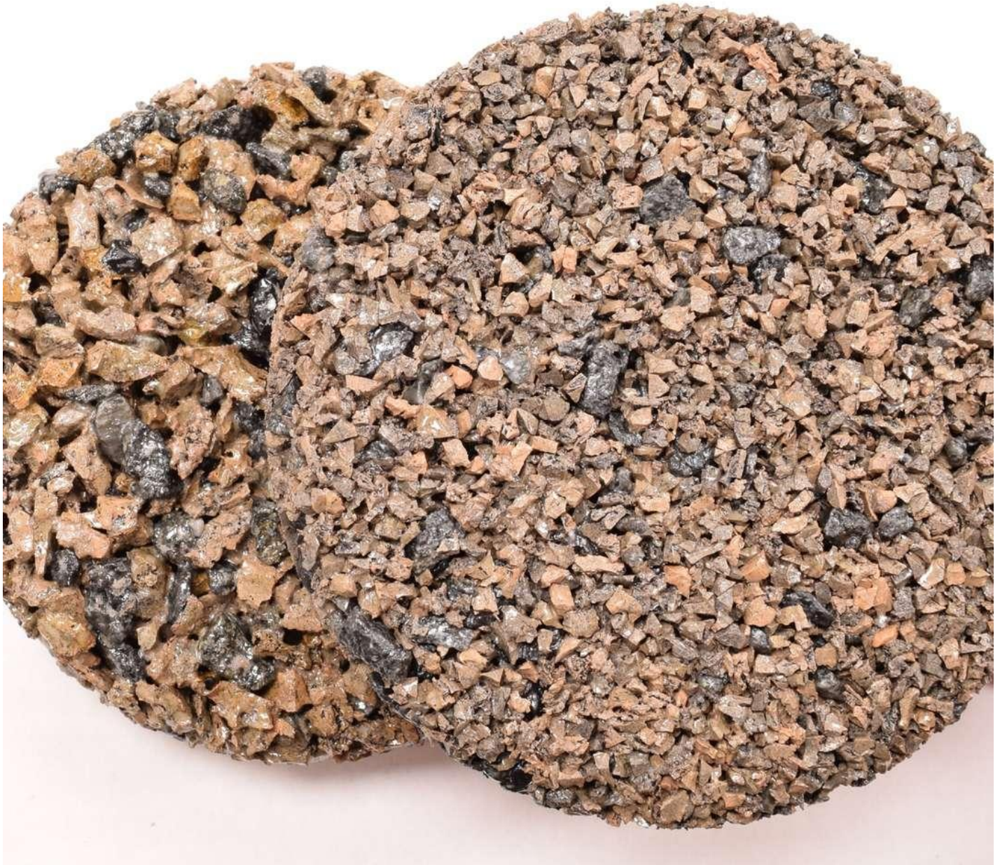
A comparison of Porous Pave's original pour-in-place permeable paving (left) and the smoother version (right).
