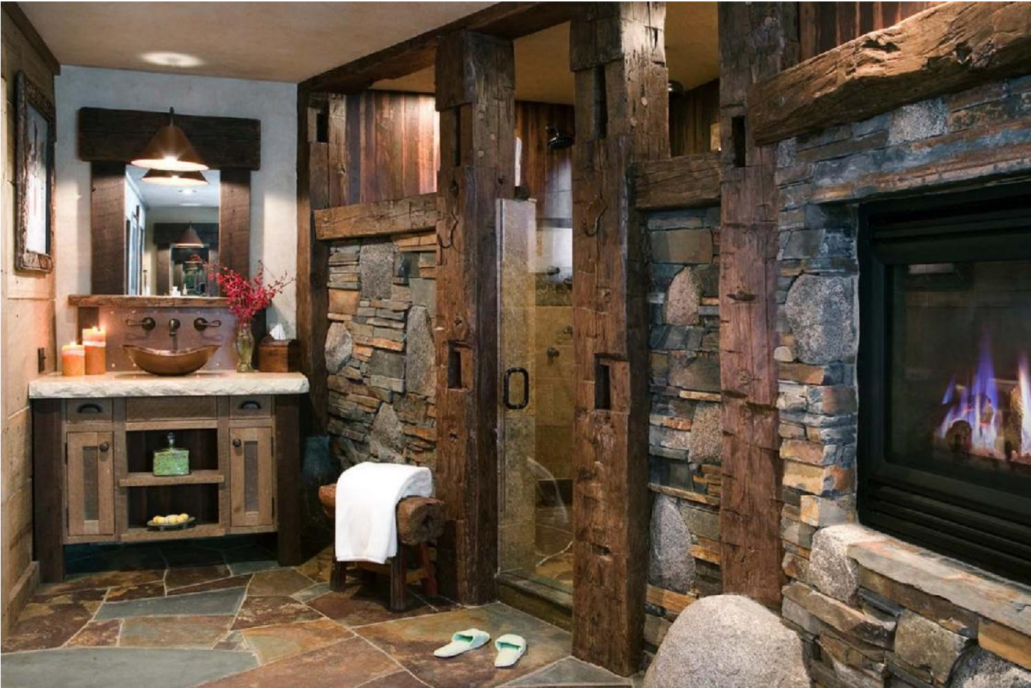
Above: The flooring is Sierra Antique Random Slate, while the stone on the walls is The stone on the walls is solid stone. Its a combination of slate flagstone, slab, and stacked stone. The beams are reclaimed timbers from old barns, adding to the rustic appeal by bringing the outdoors in.
